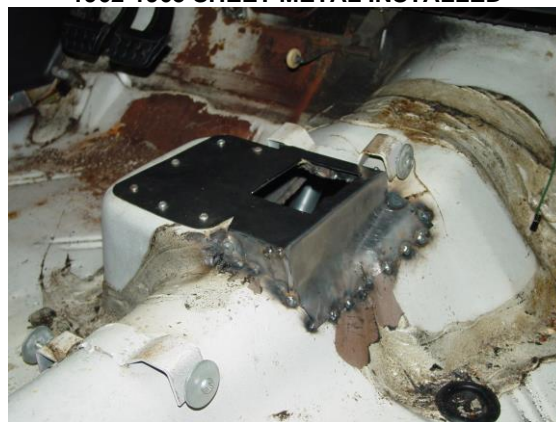
1962-1965 SHEET METAL INSTALLED
