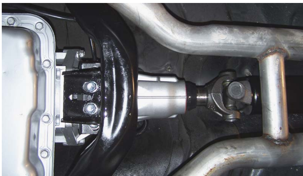
BOTTOM VIEW OF MODIFIED CROSSMEMBER AND MOUNT IN THE COMPLETED FINAL INSTALLATION.
