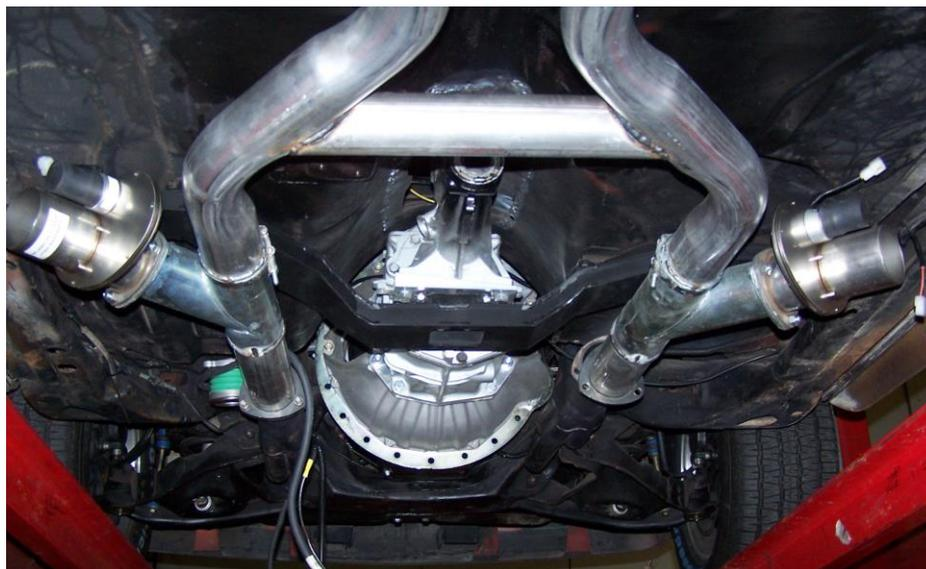
13. The rubber tailshaft sleeve may be removed at this point. Install driveshaft by inserting the slip yoke into the rear of the transmission first. Then position the rear U-joint in the differential U-joint saddles. It may be helpful to be able to turn the rear wheels. Install rear straps and torque to factory specs: 17 lb.-ft. for 1310/1330 U-bolts; 24 lb.-ft. for 1350 U-bolts (excessive torque can distort bearing cap leading to premature failure). Double check your assembly.
