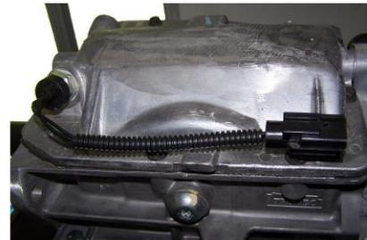
17. The reverse light switch is a black-bodied switch with (2) studs located on the driver's side of the case. The switch is a normally open, non-directional switch that will complete the lighting circuit when the transmission is in reverse. SST has provided a two-wire harness with your kit that will attach to the 5-speed reverse light switch. It can be spliced into your car's wiring harness in place of your original switch that was mounted to your 4-speed shift linkage.
