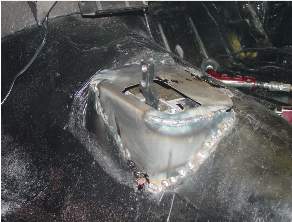
Fig. A - Sheet metal formed and welded to factory hump
