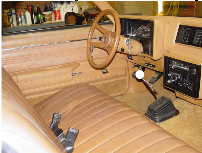
FIG. C - New boot and trim ring installed
