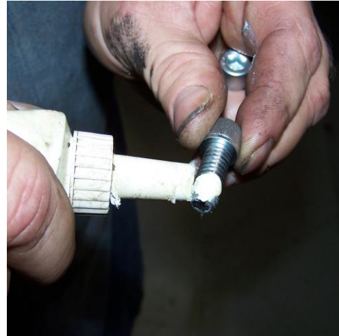
FIG. D APPLY THREAD SEALANT
