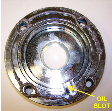
FIG. C APPLY RTV GASKET MAKER
