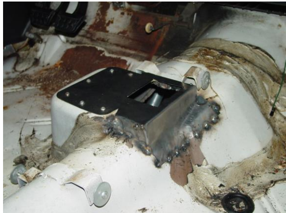
1962-1965 SHEET METAL INSTALLED
