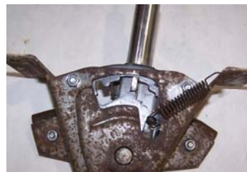
Slapstick guide and gate installed
