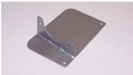
Heat shield made to bolt to exhaust header flange
