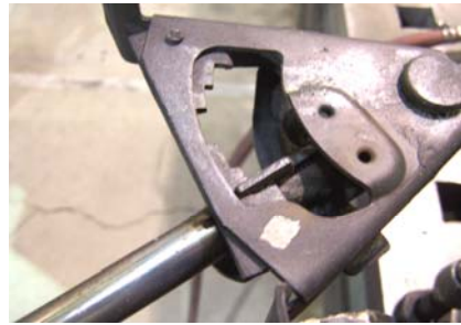
Grind off 2 rivets (driver side)
