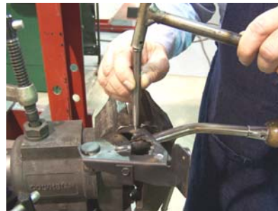
Punch rivets through
