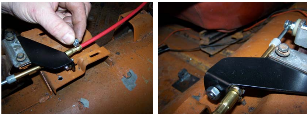
Cable tab is bolted to back side of bracket as shown
