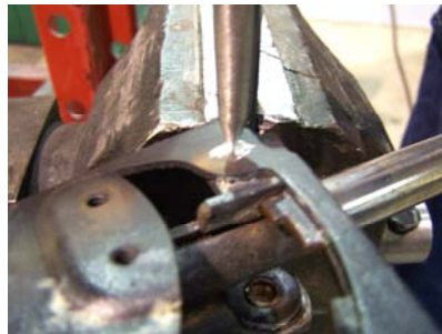
Align punch with rivet center
