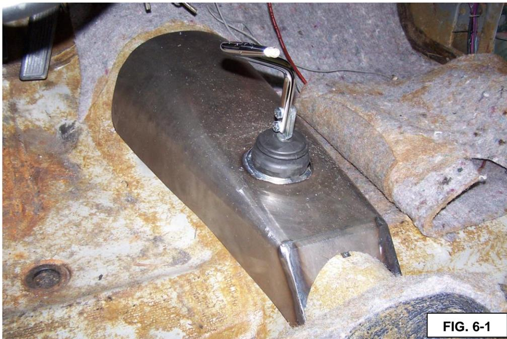
6. Apply body sealer LORD® Fuser 803DTM Metal Sealer or equivalent around perimeter joint on all body metal to prevent water intrusion. Paint exposed sheet metal surfaces for corrosion protection.
