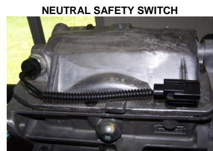
21. The reverse light switch is a black-bodied switch with (2) studs located on the driver's side of the case. The switch is a normally open, non-directional switch that will complete the lighting circuit when the transmission is in reverse. SST has provided a two-wire harness with your kit that will attach to the 5-speed reverse light switch. It can be spliced into your car's wiring harness in place of your original switch that was mounted to your 4-speed shift linkage.
