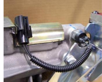
18. The reverse light switch is located on the driver's side of the main case and is a black-bodied switch with (2) studs. The switch is a normally open, non-directional switch that will complete the lighting circuit when the transmission is in reverse. SST has provided a two-wire harness with your kit that will attach to the 5-speed reverse light switch. It can be spliced into your car's wiring harness in place of your original switch that was mounted to your 4-speed shift linkage.
