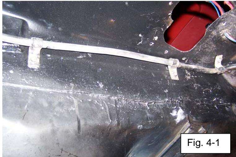
6. 1968-'75 Factory Manual cars came with a hole cut into fiberglass tunnel for manual shifter - but an additional area of tunnel must be removed to provide clearance for the T56 Magnum shift tower.
