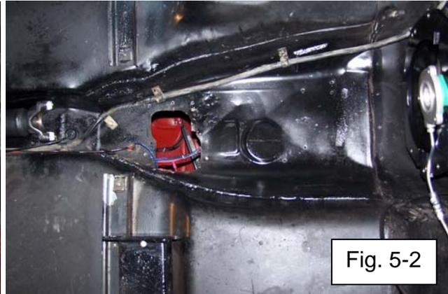
8. Because the T56 Magnum transmission is much longer than original manual transmission and the slip yoke will now be located closer to rear where the tunnel begins to taper down in width, the passenger side of tunnel wall might need to be modified for driveshaft slip yoke clearance.
