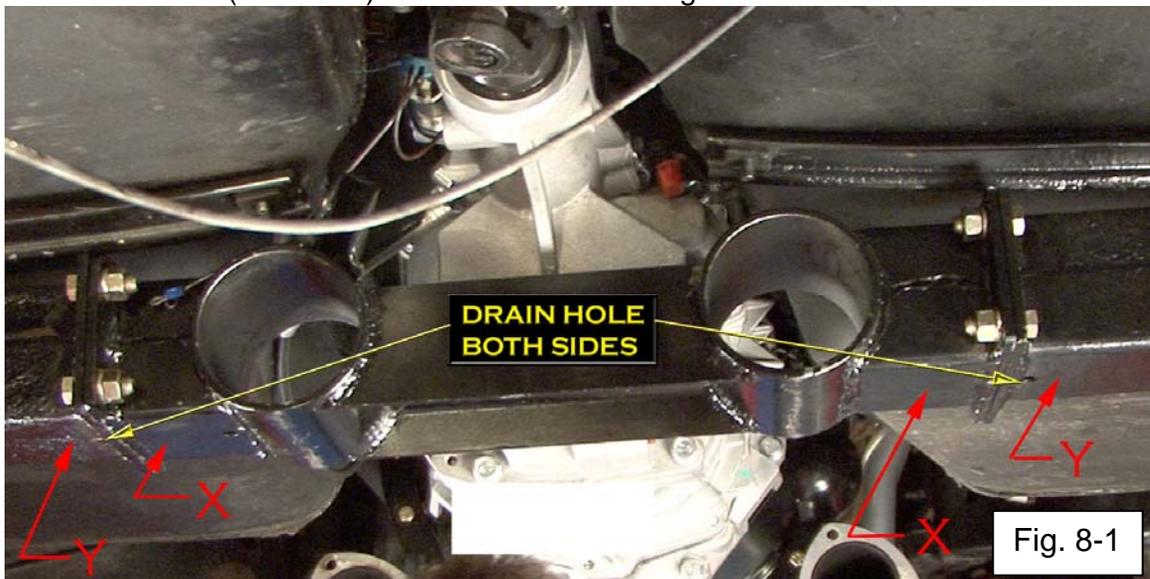
15. Tack weld the bottom, front and back surfaces of outer flanges to the cut ends of crossmember on both sides.
