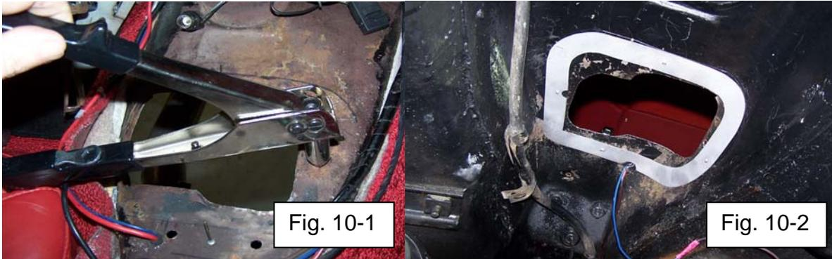
20. For 1976-'79 Factory Manual car with steel tunnel, the backing plate is not required and the BMG-03002/BMG-03102 patch panel will attach directly to tunnel with sheet metal screws. Pop rivets will NOT be used.
