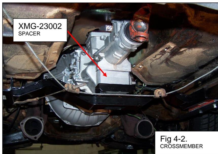
8. Install new crossmember to isolator mount with hardware pack HWG-PACK B. Raise engine until ends of crossmember are in contact with bottom surface of frame rails. Making sure crossmember is square to driveline and using the crossmember mounting holes as a guide, mark locations for new frame rail holes if required.
