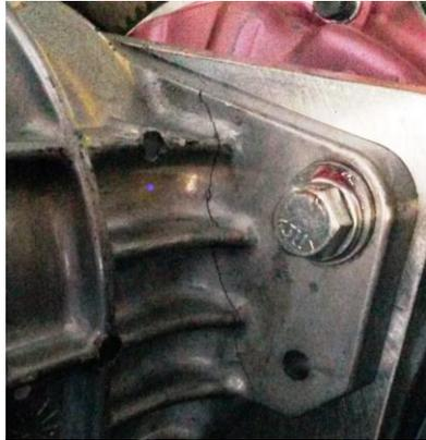
10. Once the transmission is fully seated by hand against the bellhousing, fasten with 1/2" x 1-3/4" bolts and lock washers provided (HWG-PACK A) and torque to 50 lb.-ft. Due to the tight clearance around the upper right transmission to bellhousing bolt, a socket head bolt (provided in hardware pack) can be substituted for the hex head bolt if you do not have a suitable wrench.
