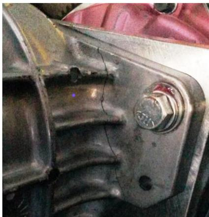
12. Once the transmission is fully seated by hand against the bellhousing, fasten with 1/2" x 1-3/4" bolts and washers provided (HWG-PACK A) and torque to 50 lb.-ft.
