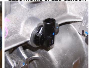
31. The electronic speed sensor is on the passenger's side of the tailhousing, just above and forward of the transmission mount pad. The sensor is a standard (2) wire GM, sine wave output, with 17 pulses per output shaft revolution, which equates to roughly 33,000 to 60,000 pulses per mile depending on axle ratio and tire size. For reference, a 26" tire with a 3.07 gear will produce 40,507 pulses per mile.
