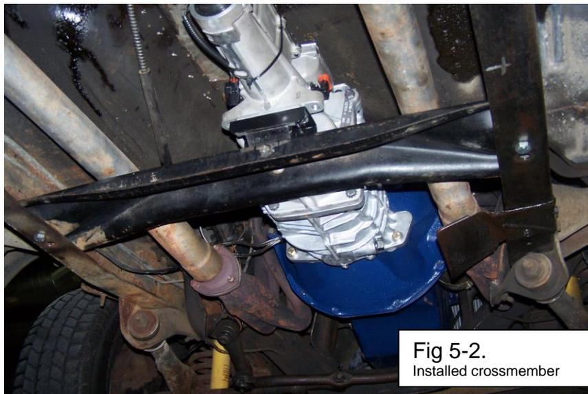
8. Verify 1/8 to 1/4" minimum clearance between TKO and tunnel. An easy way to check areas that you cannot see is to use a length of rubber hose that is 1/4" outside diameter. Loop it over the transmission at the bellhousing and see if you can slide it all the way to the tail housing. If the transmission has less than 1/4" clearance at any point in the tunnel, you may be able to "massage" the tunnel with a hammer and dolly to prevent cutting the tunnel.
