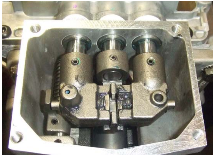
All shifter lugs installed
