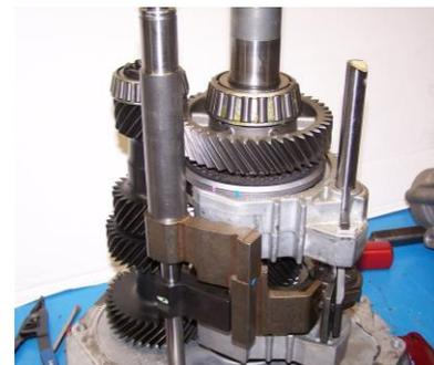
11) Set the main case into position over the output shaft and countershaft, and let it rest on top of the dowels, about an inch away from the transmission front adapter plate.
