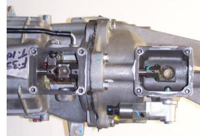
18) There are two different sized rear shifter opening cover plates included in your kit. Select the appropriate size cover for your transmission. Apply a bead of gasket sealant around the shifter opening on the transmission, and install the new rear cover using the shorter bolts supplied with kit. If desired, affix the "STX" shifter badge to the new cover plate.
