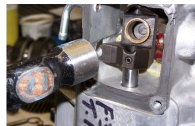
16) Install the new shifter assembly to the transmission using the (4) longer bolts supplied with kit and torque to 11-18 lb.-ft.
