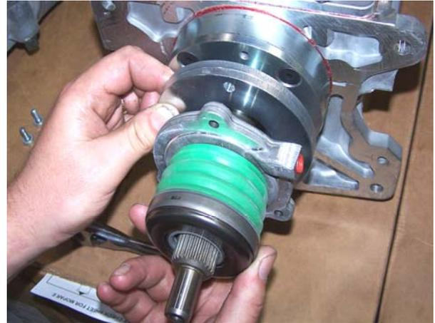
If your cushion measurement is **LESS** than 1/8", you will need a bellhousing spacer to move the transmission and CSC further away from the engine block. The spacer is 1/4" thick, and gets sandwiched in between the bellhousing and the transmission. You can only use one bellhousing spacer. If you need more than 1/4" to get your cushion within specs, you may have to resurface the flywheel, change to a thinner flywheel, or change to a different clutch.
